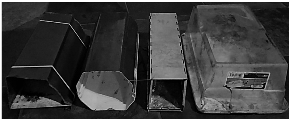
Figure 2. Four box designs for collecting tracks of New Mexico jumping mice on the Apache–Sitgreaves National Forests, Arizona, USA, during June–August 2015. Designs included (left to right) a K-style gutter with acrylic base plate, a double U-style gutter tube, a small folding Sherman trap, and a plastic modified shoebox. The modified shoebox was the most efficient and effective design.
