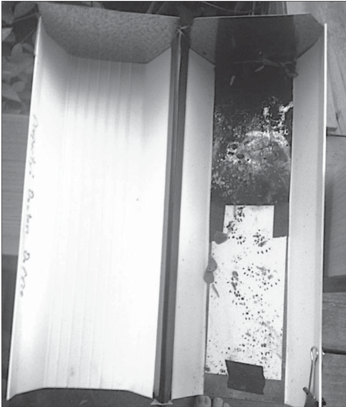
Figure 2. Track-tube design used for sampling small mammals for comparison with Sherman live trapping at 37 Alabama and Tennessee study sites, 2015–2016. Design was based on Glennon et al. (2002) but modified to reduce effects of rain splatter and feeding debris by capping one end with metal flashing and duct tape. Cotton Rat tracks are visible on the track plate.
