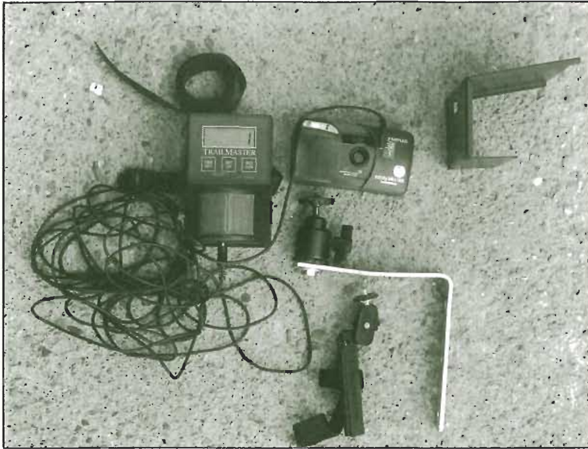
Figure 3 —The Trailmaster TM500 dual-sensor camera system. From left to right: dual-sensor unit, camera, and metal camera shield. Immediately below the camera is a ball-and-socket head bolted to a metal L-bracket for attachment to a tree; below that is the “tree-pod” that comes with the system. The camera is attached to the receiver with an 8-m wire.
