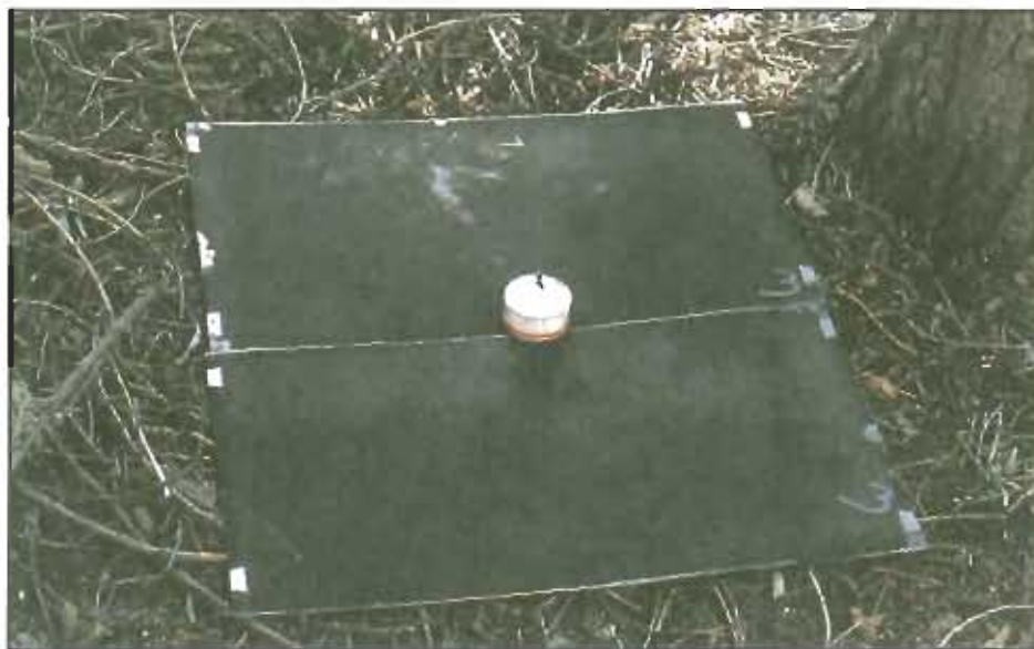
Figure 7 —Unenclosed large, sooted track plate in field, with perforated tuna can as bait.
