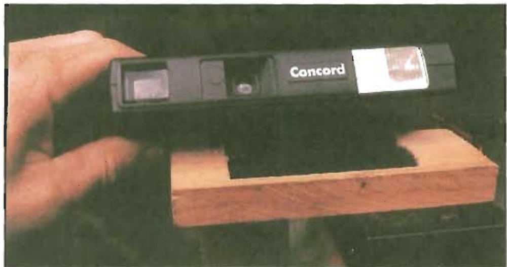
Figure 4—110 camera, raised from platform to view Velcro attachment.
