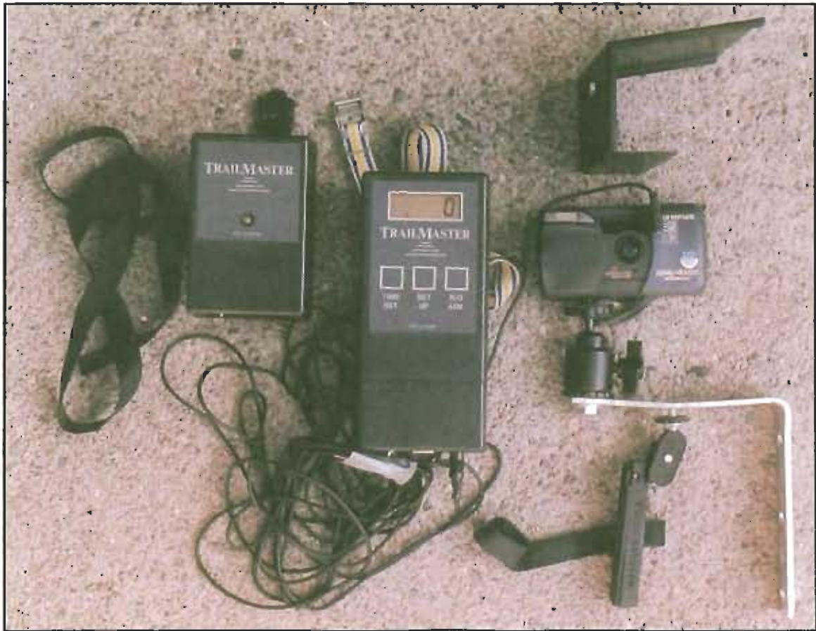
Figure 1 —Single-sensor equipment. From left to right: transmitter, receiver, and camera. Above the camera is the metal shield that protects it. Immediately below the camera is a ball-and-socket head bolted to a metal L-bracket for attachment to a tree; below that is the “free-pod” that comes with the system. The camera is attached to the receiver with an 8-m wire.
