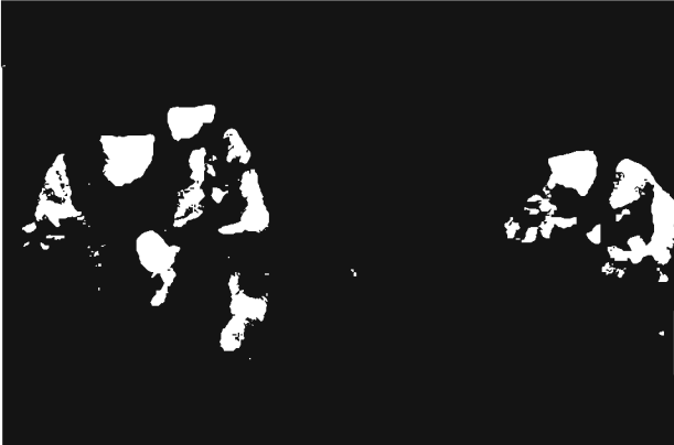
FLIR images of armed soldiers in thin foliage. Note brightest thermal images from exposed faces and hands.
