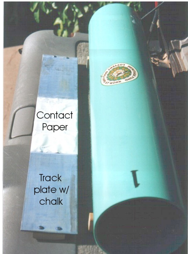
C. Track plate painted with chalk and partially covered with contact paper, along side of track station.
