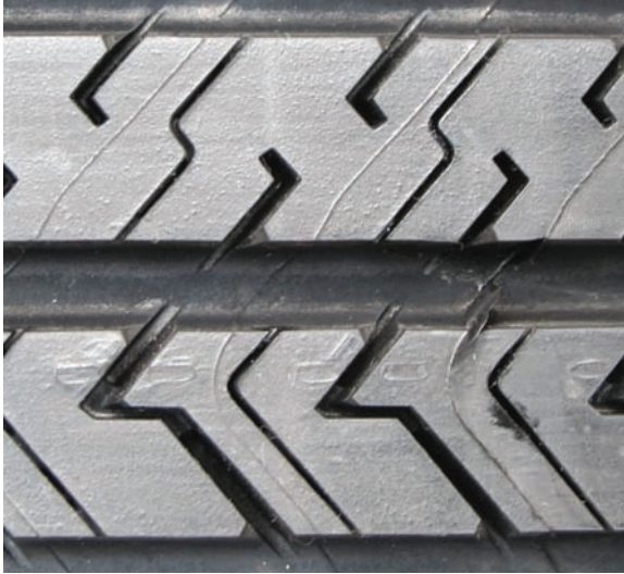
Figure 8.7. A close-up view of a small section of new tread with tapered groove bottoms, slots, and sipes.
