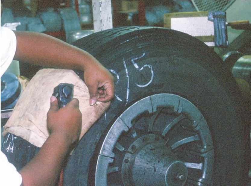
Figure 6.9. The wicking cloth is applied and stapled over the spliced area.
