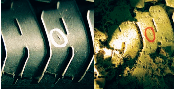
Figure 10.19. A cut on a tire and the resulting clear cut in the impression recovered by the cast.
