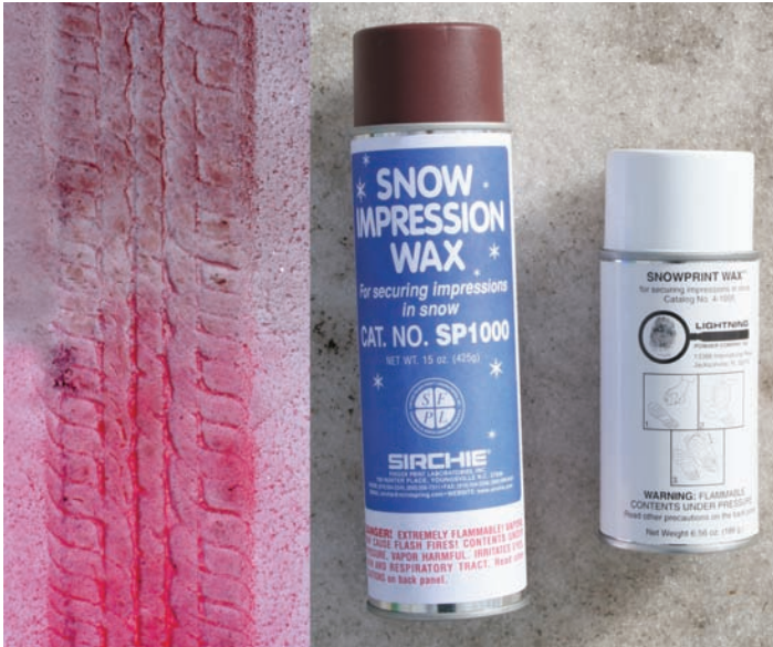
Figure 3.28. There are currently two choices of colorized snow wax, one with a brownish color (Snow Impression Wax) and one with a red color (Snowprint Wax). On the left is a tire impression in snow that has been highlighted with each.
