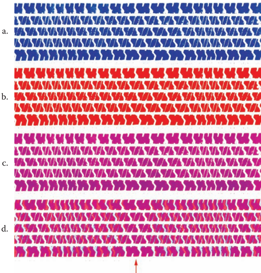
Figure 10.6. A section of one inked impression (A) and a section of the second inked impression (B) from the same tire. When one is superimposed over the other running in the same direction, they correspond perfectly (C), but when one is placed over the other in the opposite direction, they do not superimpose (D). This means this tire has directional noise treatment, i.e., the pitch sequence on one side of the tire is different than on the other side.
