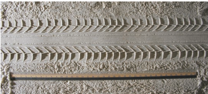
Figure 3.12. A 3-foot yardstick has been recessed into the ground to the same level (plane) as the bottom of the tire impression. This provides a properly positioned flat and rigid scale that can be used to produce accurate natural size enlargements for later examination with a tire.
