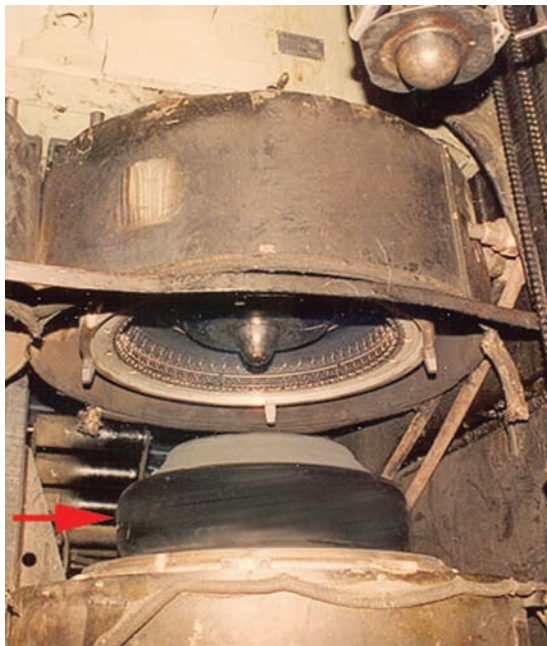
Figure 5.2B. A shell mold. The arrow points to the green tire just placed in the mold. Note that it contains no tread design. The tread design ring of the upper half of the mold is visible. The green tire is sitting on top of the bottom mold half.
