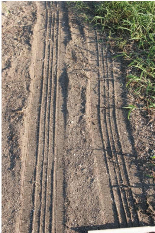
Figure 2.20. One of these impressions is straight (rear tire) and one is not straight (steering tire).
