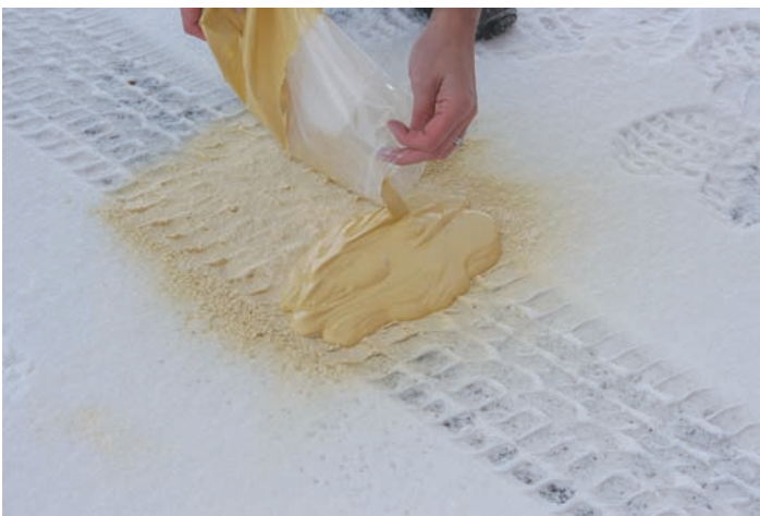
Figure 3.31. After three layers of sifted dental stone have been applied, a regular mixture of dental stone can then be safely poured over this area to complete the cast.
