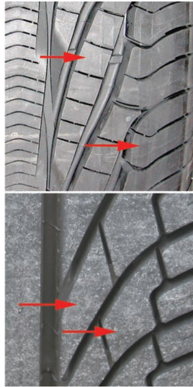
Figure 7.3. Tread blocks from two designs: the top one from a directional design tire and the bottom one from an asymmetrical design tire.
