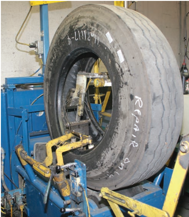
Figure 6.1. This inspection machine will help locate holes, nails, and defects that have occurred to the tire during its use.
