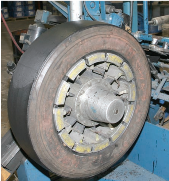
Figure 6.3. A thin layer of gum rubber has been applied around the newly prepared tire casing.
