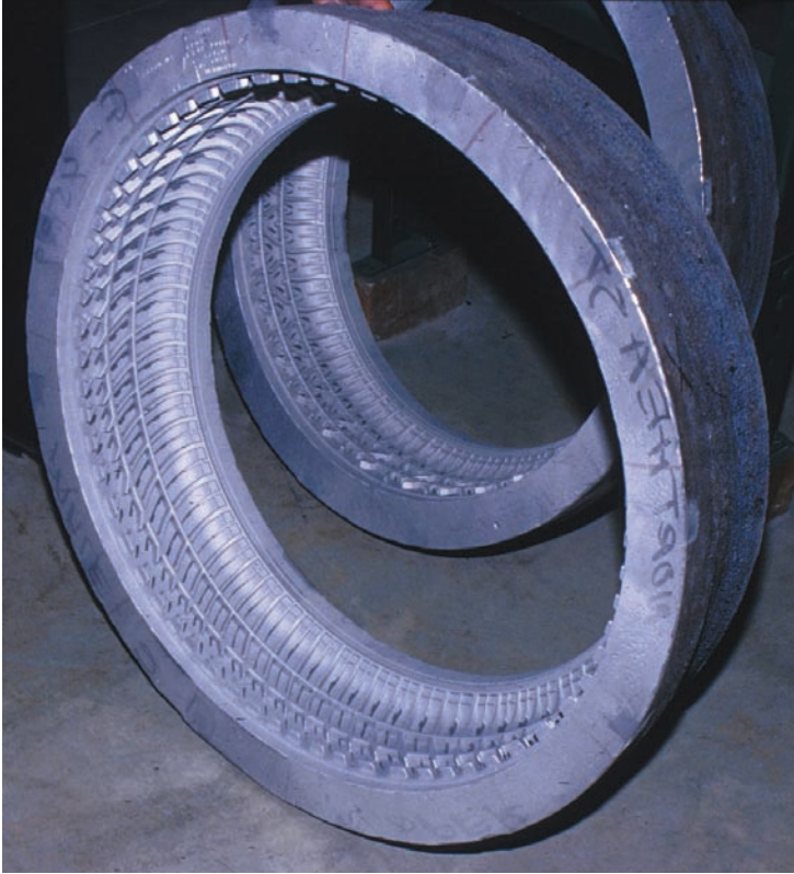
Figure 5.7. Two tread rings, each of one half of the tread design for a shell mold.
