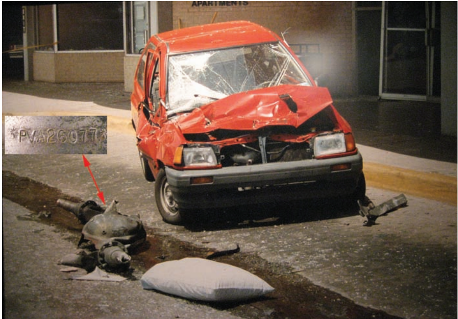
Figure 14.2. The axle from the Ryder truck, now resting on the ground and indicated by the arrow, was blown almost 600 feet into this small car, smashing its hood and windshield. A VIN on the axle allowed investigators to identify the Ryder Ford truck that was used as the bomb.
