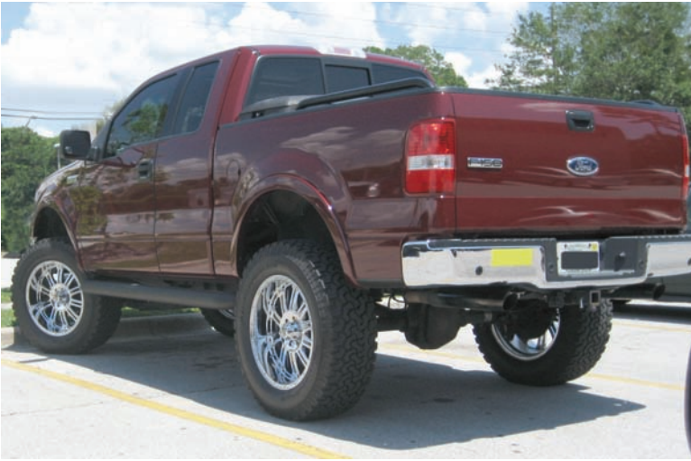
Figure 2.16. Aftermarket wheels involve wheel and tire changes that are different from the OEM equipment. All of these will likely change the track measurements.
