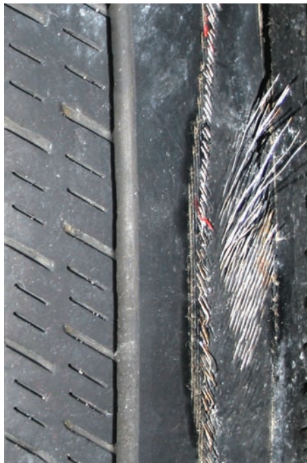
Figure 9.5. An exposed belt on a tire due to severe mechanical problems. The position and exact manner in which this belt becomes exposed and the resulting tearing of the exposed fabric and steel is random and contain numerous individual features.
