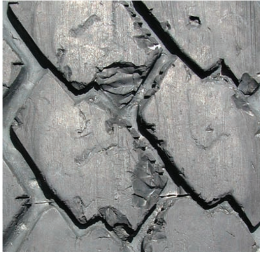
Figure 9.2. The rubber tread can get torn or ripped due to a variety of causes. This is more common in heavier vehicles and vehicles driving over poor surfaces.
