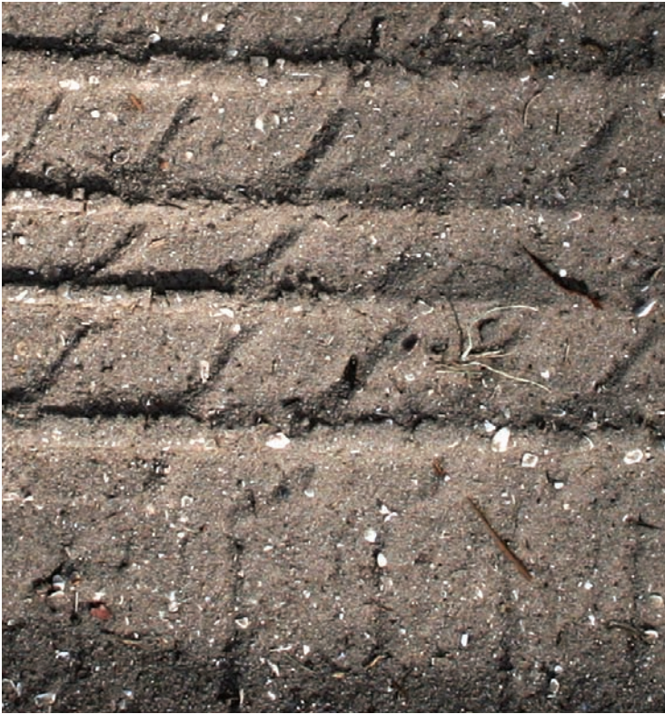
Figure 8.13. Dry soil will often fall back into the impression, partially filling the sipes and grooves of the impression, restricting detail and also misrepresenting tread depth.
