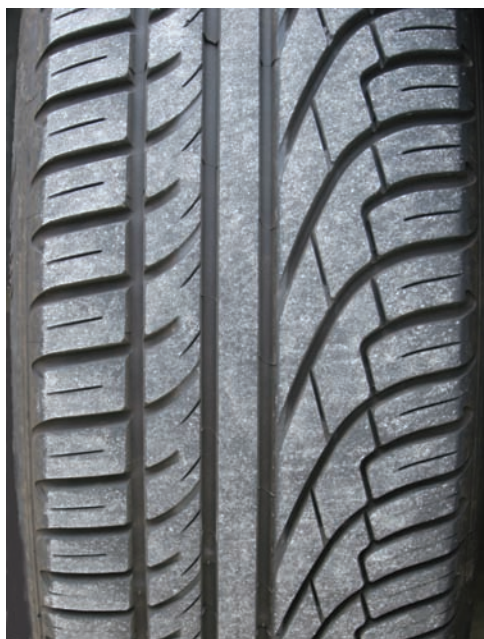
Figure 7.11. An asymmetrical tread design. This design can still be interchanged on any position of the vehicle.
