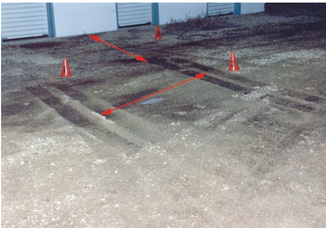
Figure 14.8. The track width measurements and the distance from the building to each point where the tracks ended were taken.
