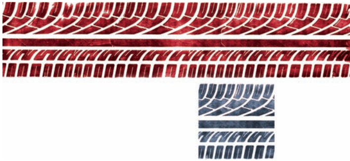
Figure 7.38. An asymmetrical tire with noise treatment but no tread wear indicator in the crime scene impression.
