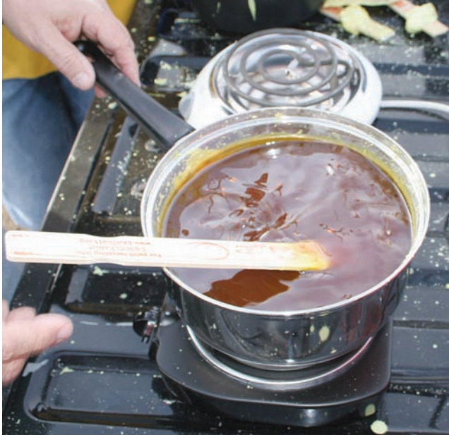
Figure 3.35. Eventually all of the sulfur will melt. Additional sulfur can then be added until the quantity needed is melted.
