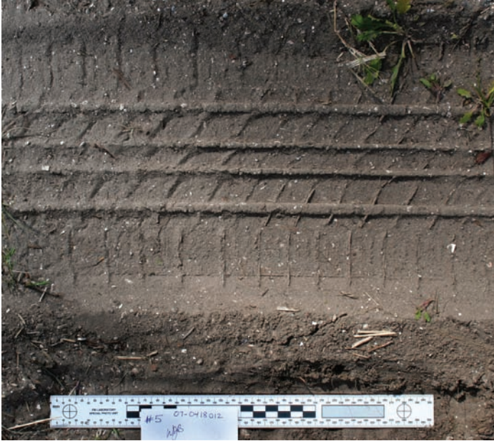
Figure 3.8. An examination quality photograph taken of the impression in Figure 3.8. This type of photograph is taken strictly for examination with a tire from a suspected vehicle. It is taken with the camera on a tripod and always using a scale that has been placed parallel to and at the same level as the bottom of the tire impression.
