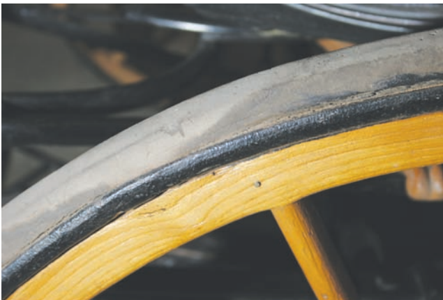
Figure 1.2. A wooden wheel covered with solid rubber on an early motorized carriage.
