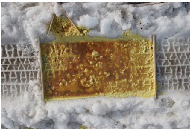
Figure 3.38. The sulfur cast after pouring. The sulfur will harden the instant it touches the snow, immediately capturing the detail of the impression. Areas of the sulfur on top will remain hot for a while until it completely cools and solidifies. A sulfur cast is extremely brittle and fragile. After it cools, a thin coat of dental stone over the back of it will help stabilize it and allow it to be preserved. When applying the dental stone, do not let any flow over the edges of the cast, as the dental stone will flow beneath the cast, undercutting it and covering the detail.
