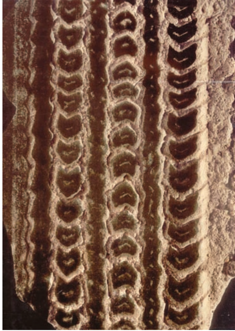
Figure 13.4. An inked impression of the BF Goodrich Belted T/A P235/70 B14 tire superimposed over the cast.
