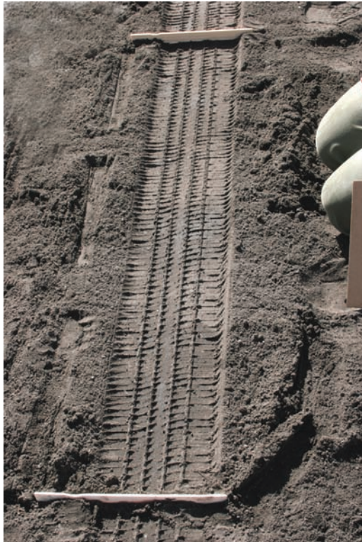
Figure 3.20. A long impression has two flat paint stirrers pressed into the soil to confine the flow of the dental stone.
