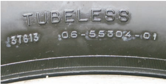
Figure 1.14. A mold number on a tire. The format of this number varies among manufacturers.
