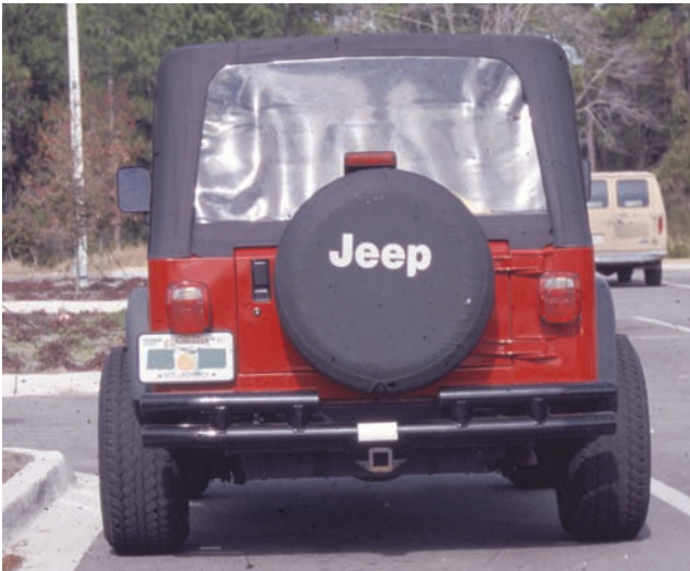
Figure 2.17. Another example of aftermarket wheels, this Jeep has oversized tires with modified wheels having a large negative offset and widening the track width.
