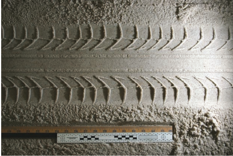
Figure 3.16. An incorrectly taken photograph where the flash was either too close to the impression or aimed improperly at the near side of the impression. The result is an overexposure at the near side and an underexposure at the far side. This is why a flash or light source must be positioned 4 to 6 feet away, allowing for the oblique light to even out.
