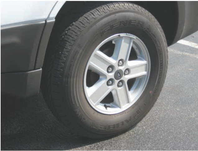
Figure 1.11B. A tire with a higher aspect ratio of 70.
