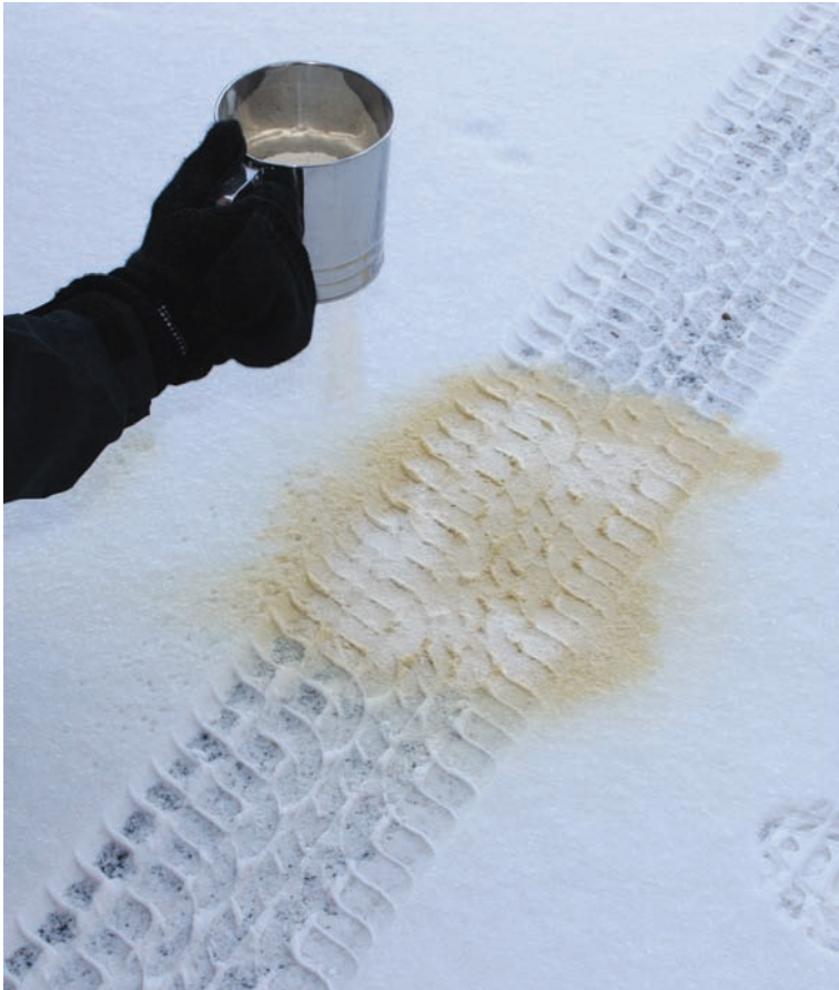
Figure 3.29. Using the dry-casting method, three separate layers of dental stone powder, each \frac{1}{8} -inch deep, are sifted over the impression. If the impression is wet or slushy snow, the powder will absorb the moisture as seen in the photo. If the snow is dry, an application of water sprayed onto the sifted powder is necessary.
