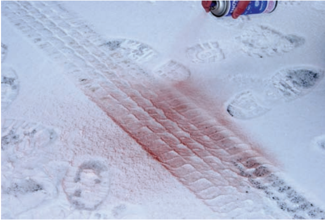
Figure 3.27. Applying a light spray of aerosol snow wax or paint is one way to highlight and increase the contrast when photographing snow impressions. The coloration of a snow impression will rapidly accelerate melting, and any impression colorized should be photographed immediately.
