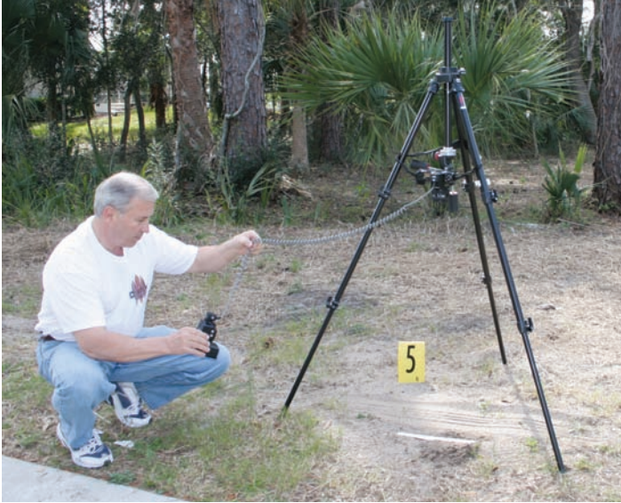
Figure 3.13. A tripod with a camera directly over the impression. A long flash cord or wireless remote flash will permit the proper use of oblique light to add contrast to the photographed impression.
