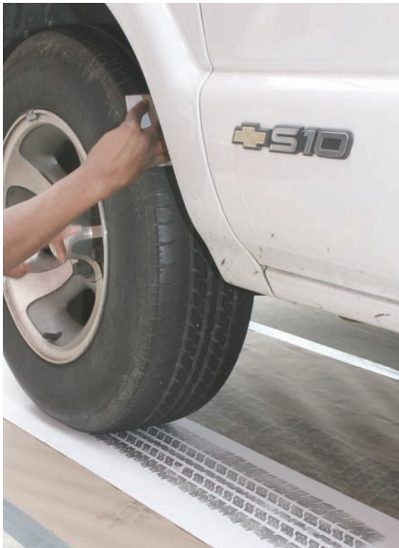
Figure 4.4. Using the Identicator Treadprint kit to obtain a known impression. The examiner uses the applicator to coat the tire with a special solution. The coated tire then leaves a detailed black impression on the treated chart board.
