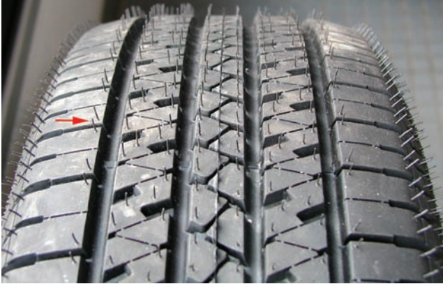
Figure 5.8. Tread molds traditionally had hundreds of vent holes drilled into the tread surface to allow for the air trapped between the green tire and the mold surface to escape. This resulted in tiny projections of rubber (arrow), simply known as vent hole rubber. With newer ventless molds, this vent hold rubber will only be found on the sidewall areas.
