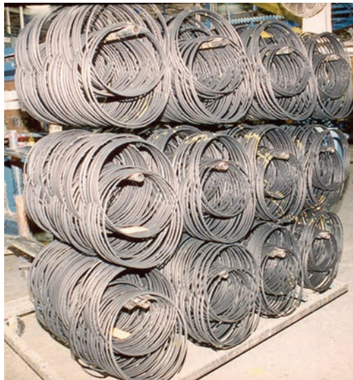
Figure 5.10. A supply of beads ready to be taken to the tire builder. The beads on each side of the tire resist centrifugal forces and help hold the tire on the rim.
