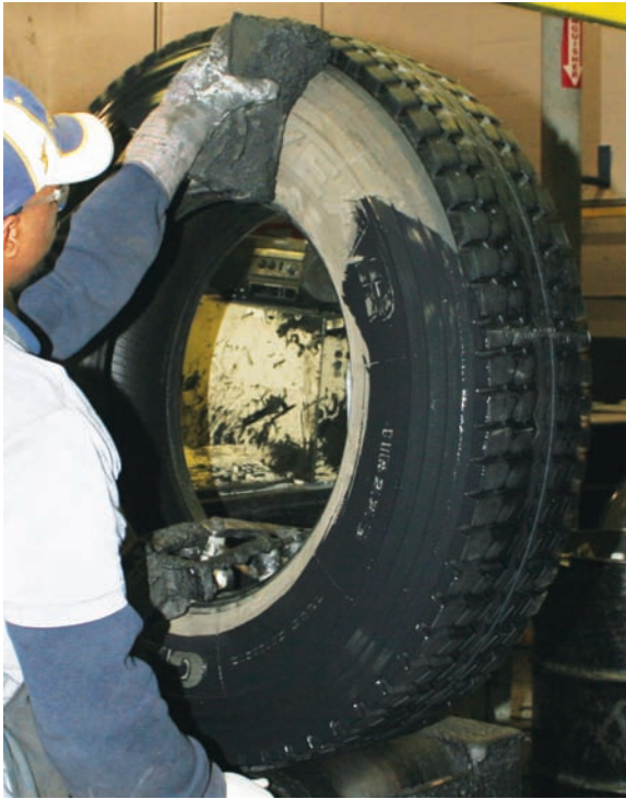
Figure 6.12. The retread process will end with the tire receiving a coat of protective paint. This is mainly for aesthetic reasons, to make the sidewall tire rubber appear new and the same color as the darker new tread but also to cover the writing that is typically placed on the sidewalls as they go through the retread process.
