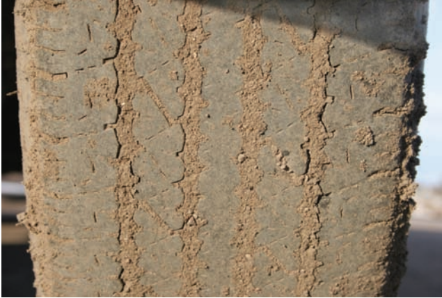
Figure 8.14. A tread caked with mud or snow cannot produce an impression that accurately replicates its actual condition of wear.
