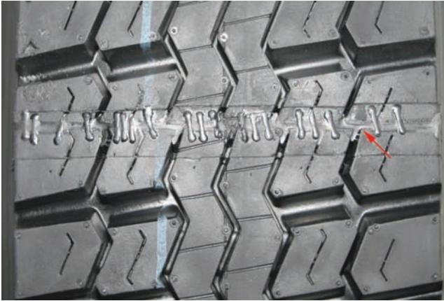
Figure 6.7. Numerous plastic staples have been used to temporarily hold the splice joint together until the tire is cured in the autoclave. The staples remain in the tread and represent additional individual features. Note the misalignment of the tread design and the extra melted gum rubber that has filled the splice area, both indicated at one point with the arrow.
