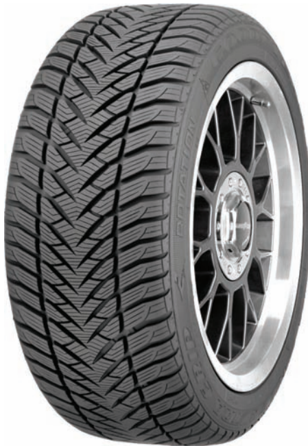
Figure 7.15. Modern snow tires look like ordinary tires but have special rubber compounds that make them perform better in icy conditions.
