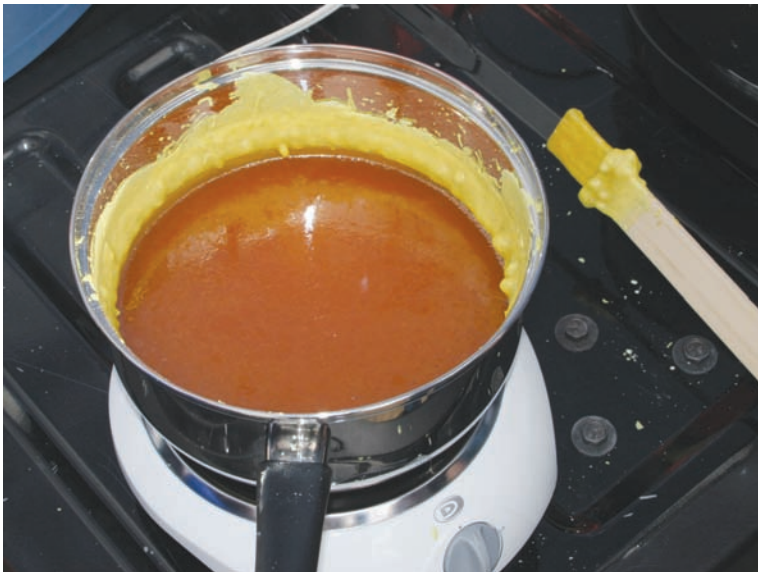
Figure 3.36. The heat is turned off and the sulfur is allowed to cool, stirring occasionally to maintain an even temperature. When the temperature of the sulfur lowers back to its melting point, it will begin to form crystals and will appear cloudy, as pictured here.
