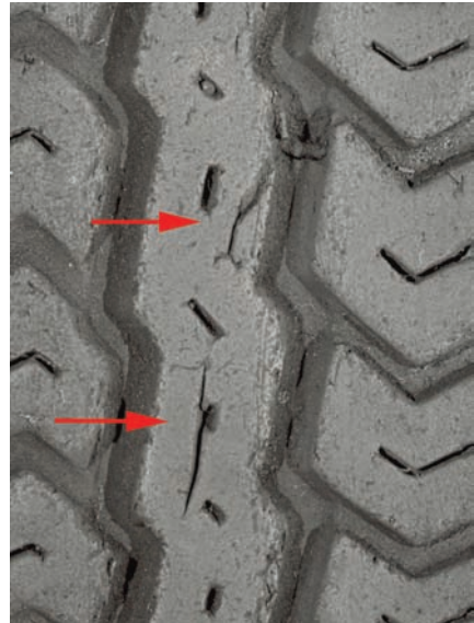
Figure 13.5. An enlarged area of the tire which contained individual characteristics also found in the cast.
