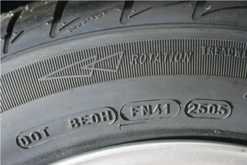
Figure 7.10. Symbols and words will denote the direction of rotation for directional tread designs.
