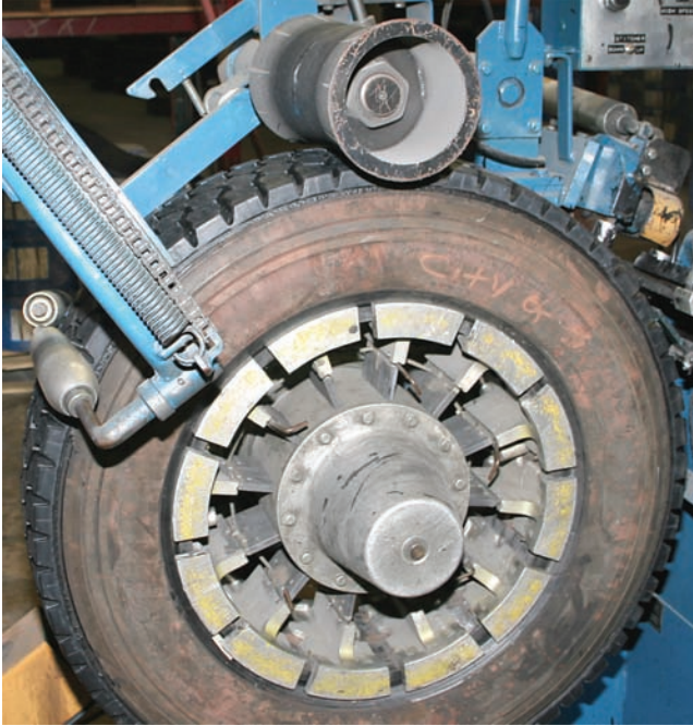
Figure 6.5. The tire revolves as the pre-cure tread stock covers the old casing. The machinery presses the new stock firmly against the casing.
