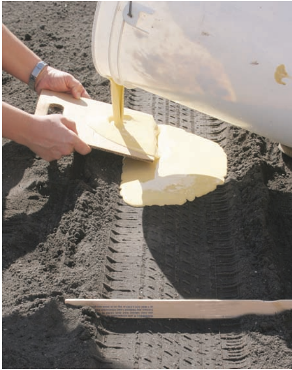
Figure 3.23. The dental stone is poured onto the center of the cardboard held close to the ground. The cardboard is tilted toward the center of the impression. The person holding the cardboard moves it up and around the impression to ensure the entire impression is filled with dental stone.
