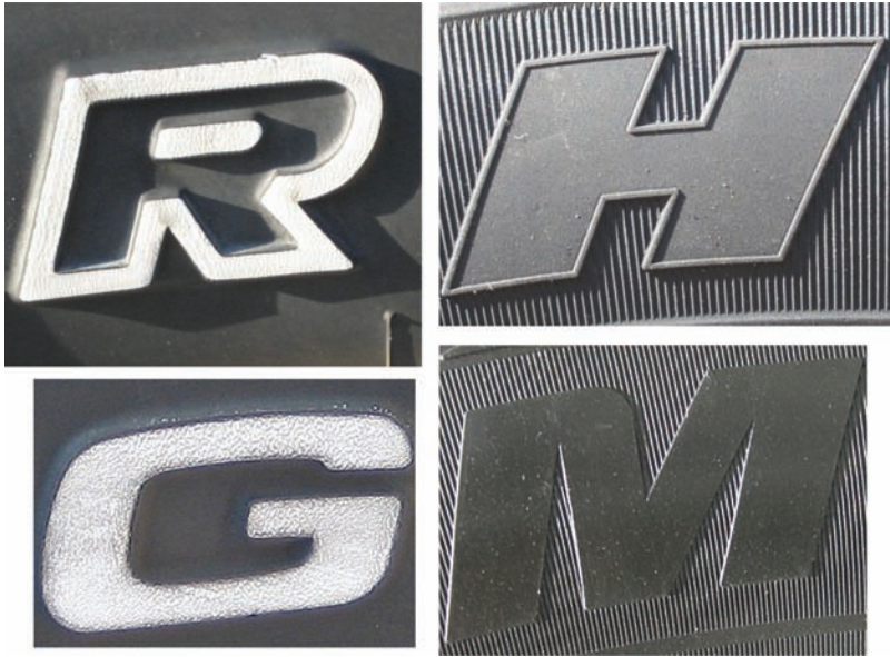
Figure 12.2B. White letters (WL) and outlined white letters (OWL) on a tire will make that tire a high-profile tire and may be of value in locating suspect vehicles in smaller cities.
