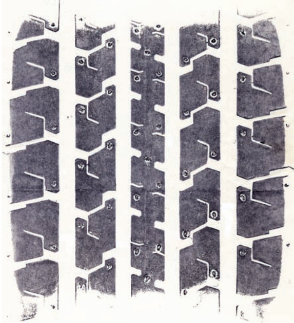
Figure 1.3. A footprint of a radial tire. The footprint is the contact area the tire makes against a hard flat surface under load.
