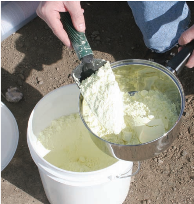
Figure 3.33. A quantity of powdered or prill sulfur is added to a pan.
