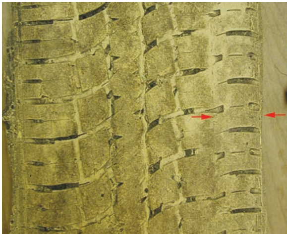
Figure 2.2. A cast taken from a scene where a small portion of the front tire impression has not been obliterated by the tracks of the rear tire. This portion is on the edge of the cast in the area between the red arrows. This is either due to the difference in track width between the front and rear tires and/or due to a slight turning of the vehicle.
