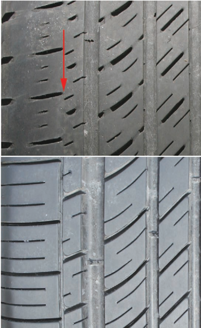
Figure 8.10. A tread that has a small groove running circumferentially around the shoulder area of the tire and a worn tread of the same design. The worn tread has resulted in the elimination of the smaller groove. Note also the changes in the small transverse grooves and sipes due to wear.
