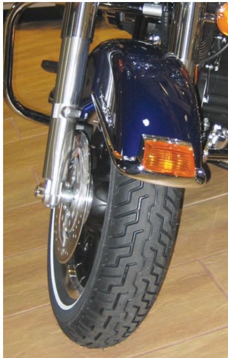
Figure 7.14. A motorcycle tire does not need varied pitch sizes, as it is not concerned with noise.
