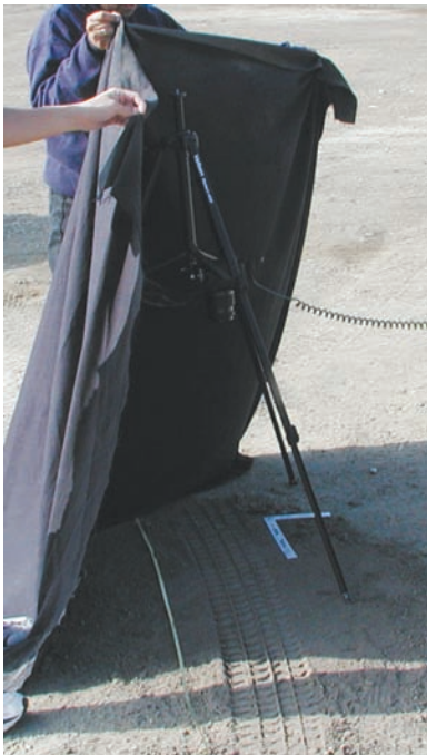
Figure 3.17. The use of a black cloth to block out bright ambient light is necessary. If this is not done, then the oblique light from the flash will be dominated by the existing bright ambient light.
