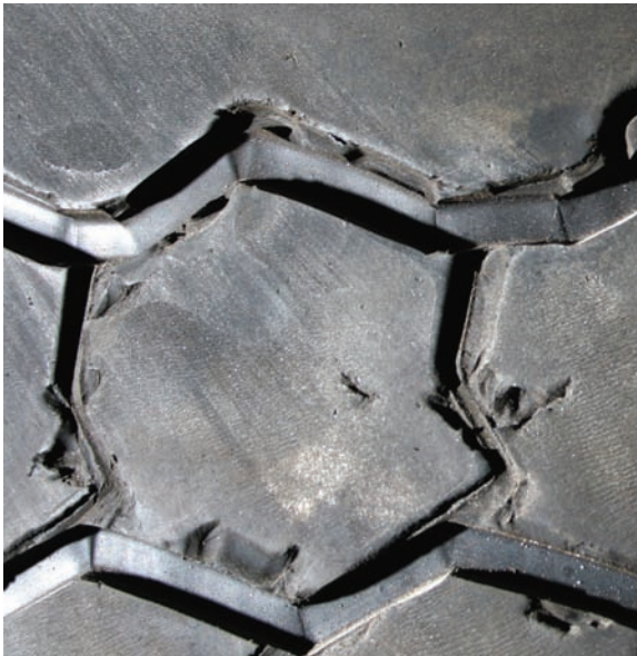
Figure 6.19. A small section of a regrooved tire shows the uneven grooving as well as many areas where the existing tread was marred, producing a large number of individual characteristics.
