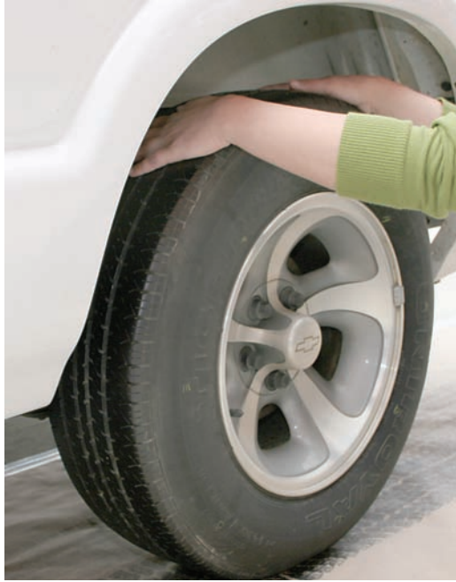
Figure 4.17. The petroleum jelly is applied evenly and with bare hands to the tread surface. This may have to be done in two or three parts to cover the entire tire circumference.
