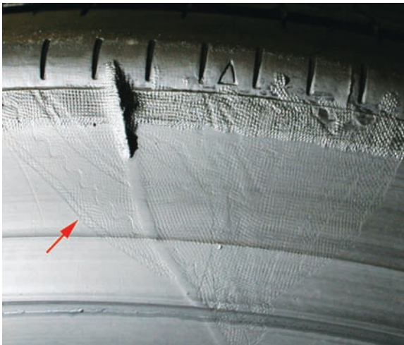
Figure 6.11. The arrows point to the transferred texture of the wicking cloth, which is placed over the splice in the pre-mold process.
