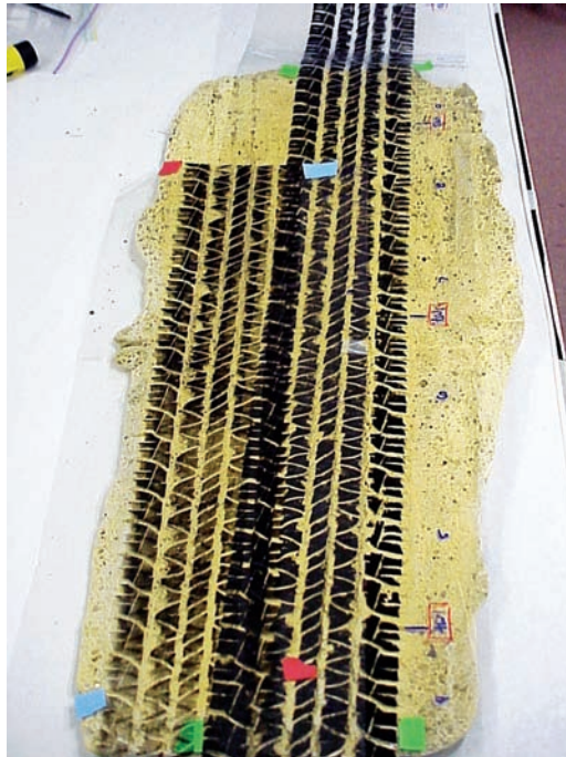
Figure 10.14. Two cast impressions with inked impressions positioned. The colored pieces of tape have been placed on the cast and inked impressions as well as the tire to help organize a systematic examination with the respective portions of the tires.
