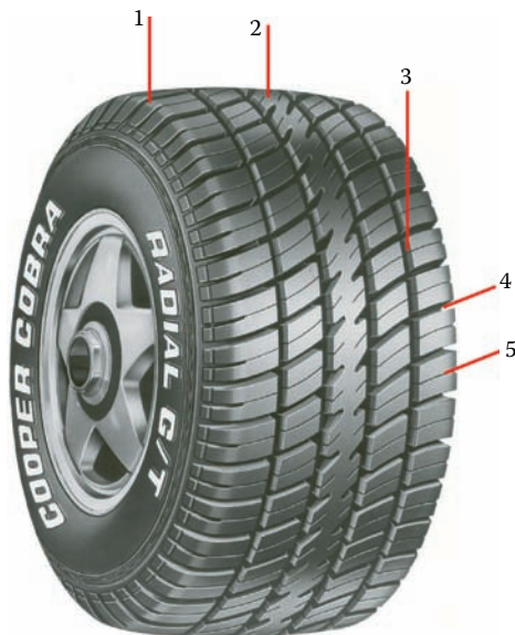
Figure 7.7. A symmetrical tire design. This design has two shoulder ribs (1); a solid center rib (2) with two divided inner ribs in between; circumferential grooves (3); lateral grooves or slots (4); and sipes (5).
