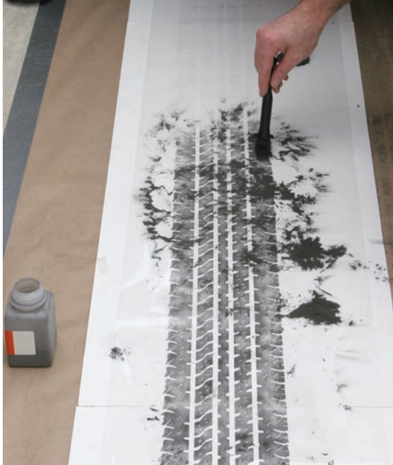
Figure 4.19. Black magnetic fingerprint powder is applied to the petroleum jelly impression on the clear film while it is still taped to the chart board. The chart board will be placed on its side and tapped to remove the excess powder. Two to three light coats of a fast-drying glossy acrylic spray will then be applied to protect the impression and prevent it from smearing.
