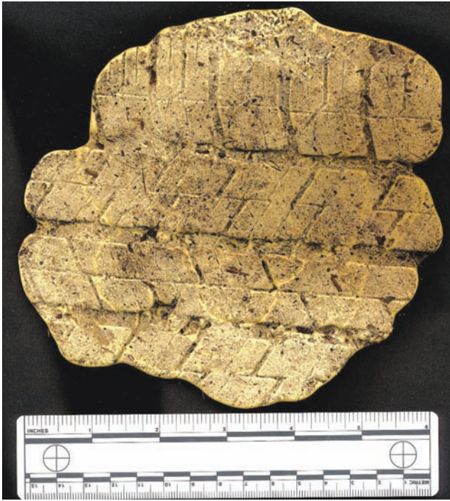
Figure 3.18. A 2-pound bag of dental stone will only produce a small cast approximately 6 inches long. This is not the proper way to cast a tire impression. A 3-foot-long tire impression will take anywhere from 12 to 25 pounds of casting material, depending on its depth and width.
