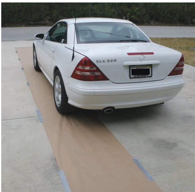
Figure 4.6. A 50-foot section of brown contractor paper has been taped to the ground to provide a clean surface. The vehicle will then be positioned at one end of the paper.
