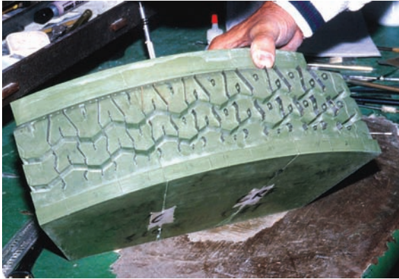
Figure 5.5. A model of tread design after insertion of the sipe blades.
