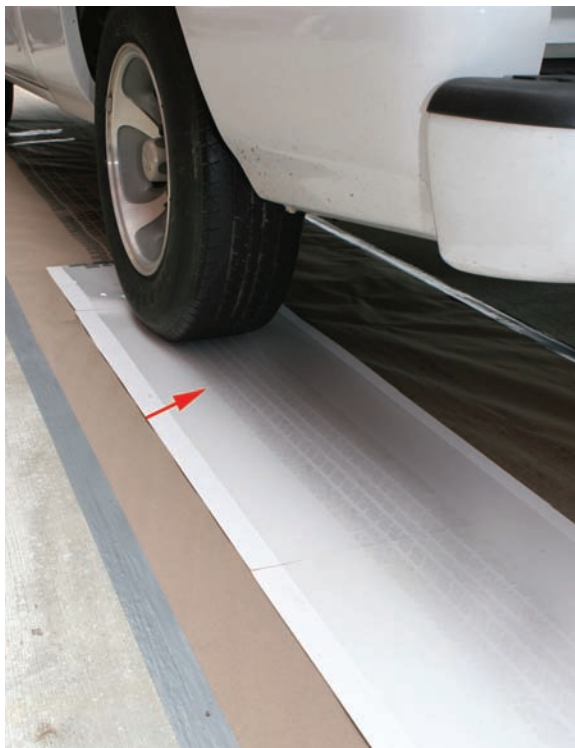
Figure 4.18. The tire leaves a very thin deposition of petroleum jelly on the clear film, seen at the arrow.
