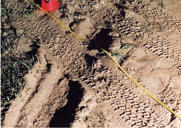
Figure 14.14. A long tape measure was laid out along the length of each separate track to help keep track of the individual examination-quality photographs taken.
