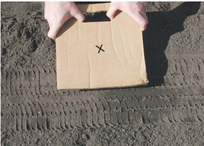
Figure 3.22. A piece of cardboard, like this dental stone box top, can be used to deflect the pressure of the dental stone as it is poured into the impression. The person pouring the dental stone should pour onto the center of the cardboard, where marked with an X.
