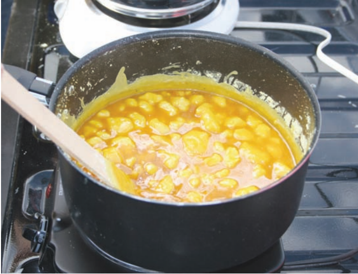
Figure 3.34. The pan is placed on to a hot plate and slowly heated to melt the sulfur. As the sulfur begins to melt, it will clump around the unmelted sulfur.
