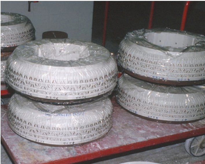
Figure 5.6. White models are prepared from the master. It is these models the molten aluminum will be poured around to produce the tread rings.
