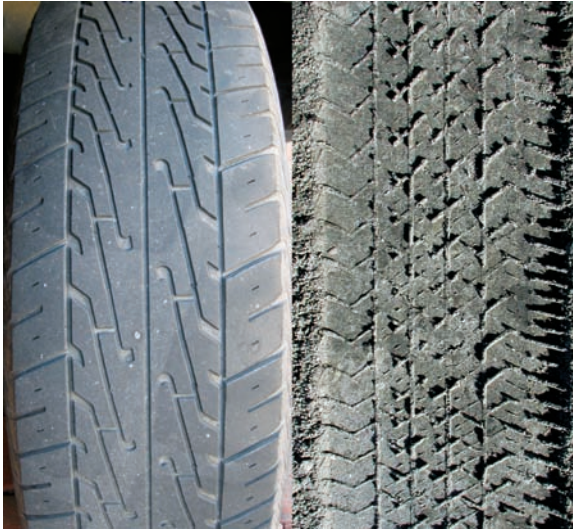
Figure 10.2. The tire on the left is clearly a different design from the design in the crime scene tire impression on the right and therefore could not have produced that impression.
