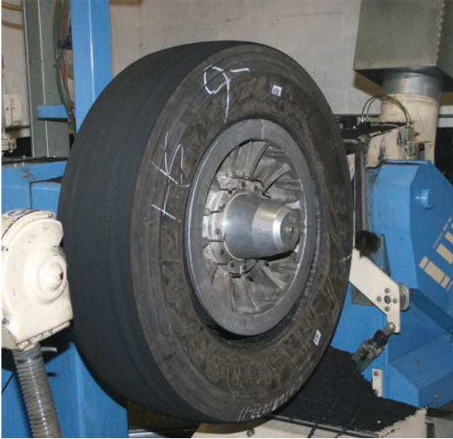
Figure 6.2. A tire on a buffing machine. The buffing machine removes the old rubber and ensures the tire surface is properly round.
