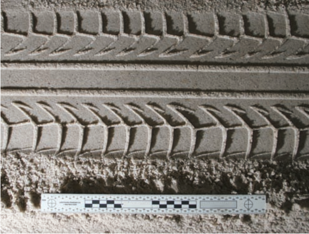
Figure 3.11. This is an example of incorrectly using a scale. The scale is resting on the edge of the impression at least a \frac{1}{2} to 1 inch higher than the bottom of the impression. This photograph will not be useful in a dimensional analysis with a known tire, because there is no way to make an accurate photographic enlargement of the impression. When the scale is enlarged to its natural size, the tire impression will not be accurately sized.
