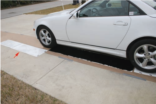
Figure 4.11. The inked board is placed between the front and rear tires so the rear tire will roll straight down and across the center of the inked surface. The other chart board, identified with the red arrow, has a piece of clear media film taped to it. As the vehicle moves forward, it must be slipped between the front and rear tires so the inked rear tire will deposit the inked impression across it.
