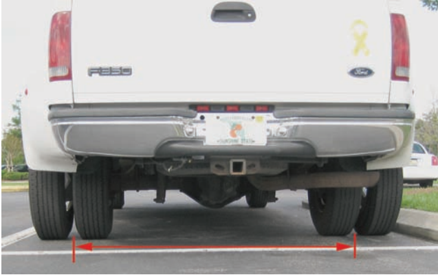
Figure 2.8. The industry track width for dual tire assembly vehicles is from the center between the two tires on one side to the center between the two tires on the opposing side of the same axle.
