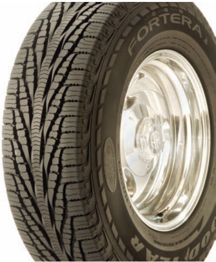
Figure 7.9. A directional tread design. This tire is made to perform best when operating in the direction indicated by arrows on its sidewall.
