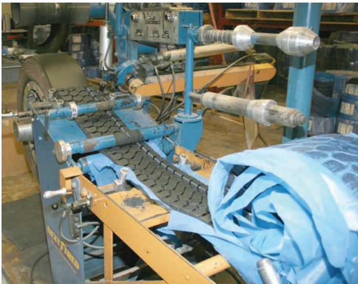
Figure 6.4. The pre-cured tread stock is fed from the roll in the foreground to the tire casing in the background. The gum rubber will cause the pre-cured tread to temporarily stick to the tire until it is cured.
