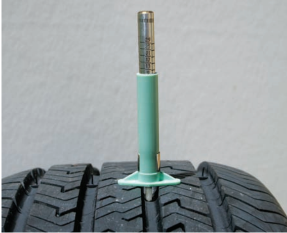
Figure 8.11. A tread depth gauge positioned on a tire. This is a plunger type of gauge with increments for each 32nd inch in depth.
