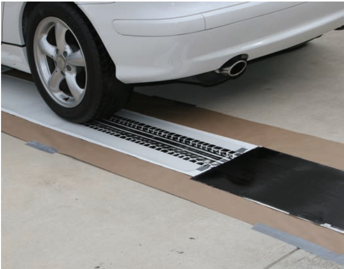
Figure 4.12. As the vehicle moves forward from the inked board onto the media film, it will leave its full-circumference impression.
