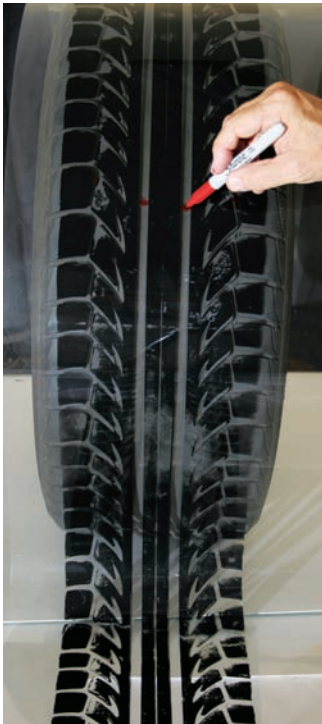
Figure 10.8. Synchronizing the inked impressions with the tire they came from, including marking the positions of each of the tread wear indicators, is part of the preparation prior to examination.
