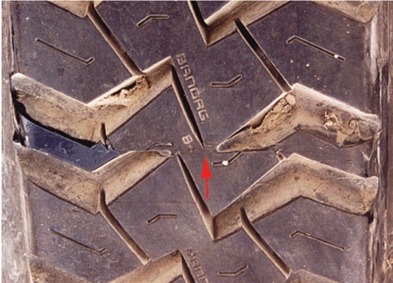
Figure 6.8. A worn retread with the typical mismatch of the design at the splice joint.
