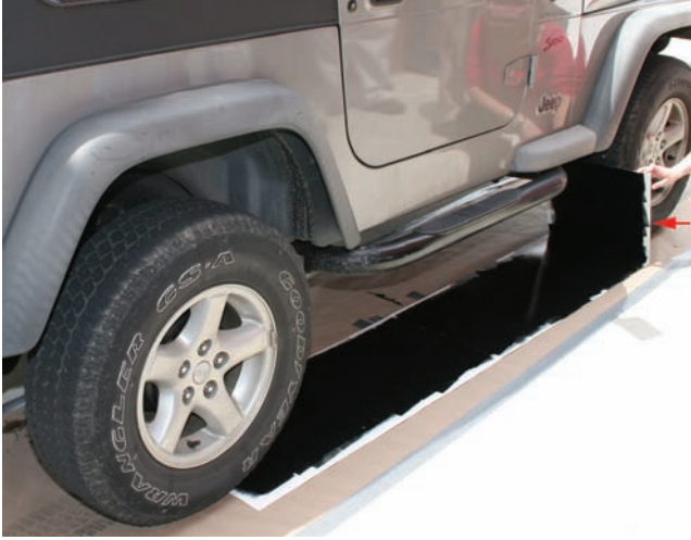
Figure 4.8. This vehicle has tires with a large circumference but a relatively short wheelbase and therefore requires the length of chart board for both the ink and film to have a hinged section at the end (arrow) so it can fit between the tires. As the vehicle moves forward, the hinged area is lowered. This will have to be done for both the inked board and the clear film that receives the impression in order to obtain full circumference impressions.
