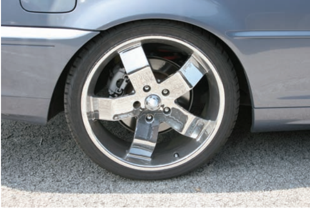
Figure 1.11A. A tire with a low aspect ratio of 35. Low aspect ratio tires appear almost flat.
