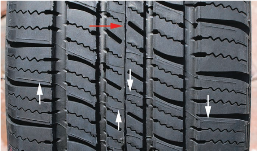
Figure 5.2C. The mold parting line of a shell mold (red arrow). The white arrow denotes the ventless seams where air escapes during mold cure. These seams end at the mold parting line on a shell molded tire.
