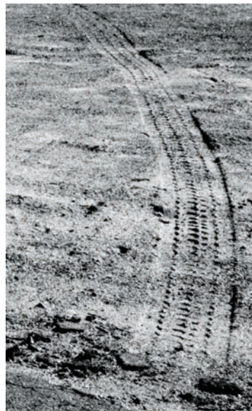
Figure 10.13. A poorly taken photograph will limit the examination of tread design and possibly prevent any meaningful examination.
