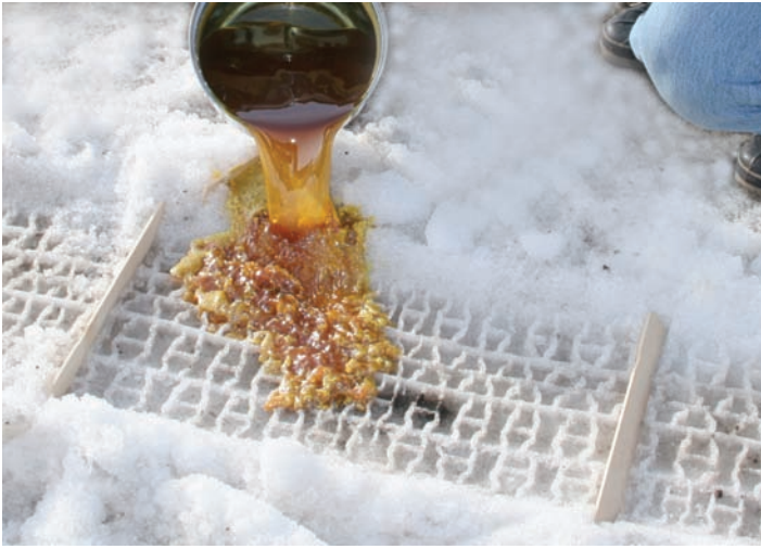
Figure 3.37. The sulfur must be poured steadily without interruption. The formation of a pathway outside of the impression that can direct the flow of the sulfur into the impression is recommended. Creating a chute with two paint stirrers or using other methods to direct the flow is usually necessary. Here the sulfur is first poured outside the impression area but is directed into the impression.
