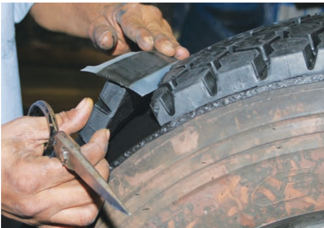
Figure 6.6. The layer of gum rubber runs around the tire casing and is the dark thin material seen here between the new tread stock and the old casing. The operator will often add some additional gum rubber to go between the splice joint.
