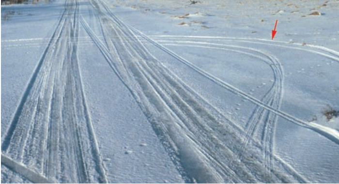
Figure 2.11. One of several photographs taken of turning tracks at a scene. Measurement of the turning diameter of these tracks will allow for inclusion or exclusion of a suspect vehicle.
