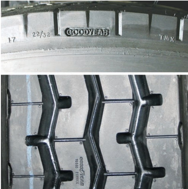
Figure 6.13. Pre-cured stock will often contain molded information on the edge such as 22/32nds, Goodyear, and TMX, which can be associated with the source of the retread stock. Other stock will have lettering or information on the actual tread surface. Both examples are seen here.
