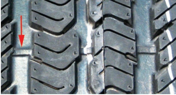
Figure 7.30. Tread indicator in a new tire is raised 2/32 inch above the groove depth.
