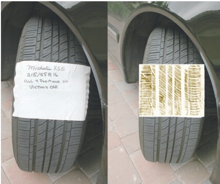
Figure 4.3. Pressing a white adhesive lift against a tire tread will provide an elimination record of a tire design. The vehicle information can be written right on the lift. On the right is the lift, turned around to show the tire design.
